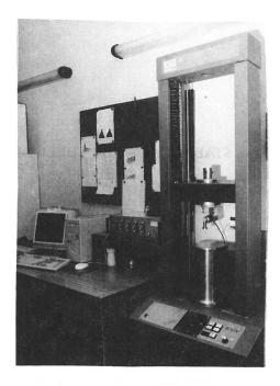
**Photo 1.** The equipment for measurement and evaluation of destructive power.
