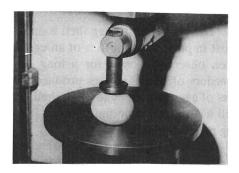
Photo 2. Measurement of the power needed for burst of egg shell.
